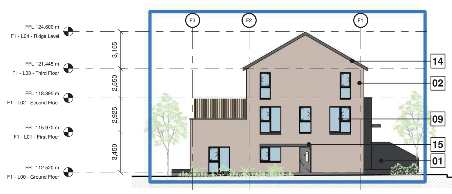
6 PROPOSED ELEVATION - BLOCK F1 - NORTH - PART V 1 : 200
