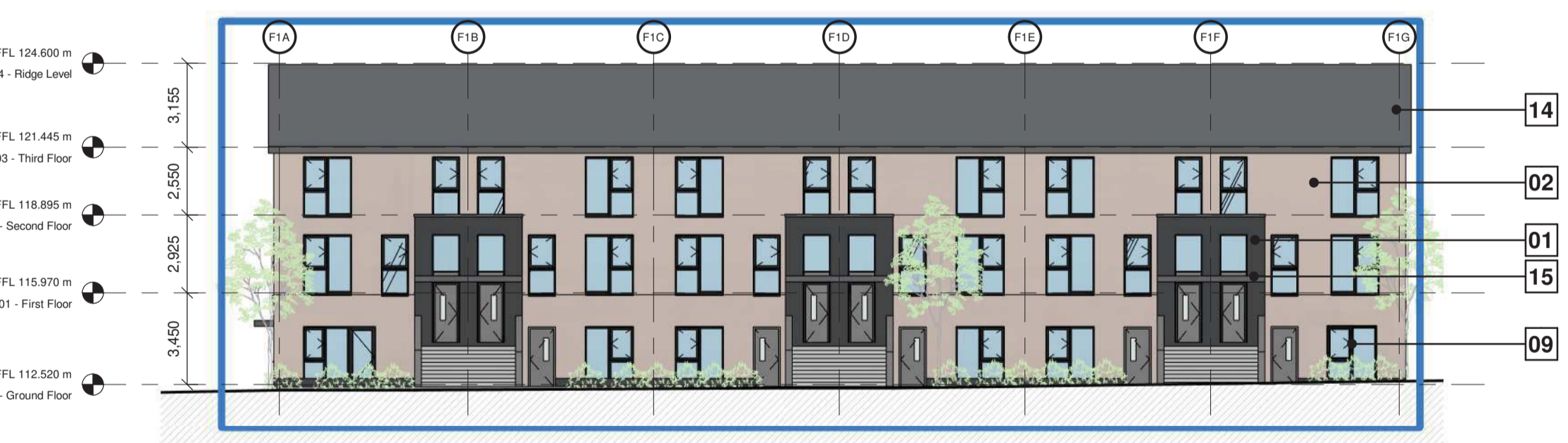
8 PROPOSED ELEVATION - BLOCK F1 - WEST - PART V 1 : 200
